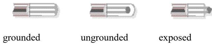
Figure 3. Different types of thermocouple junctions.
